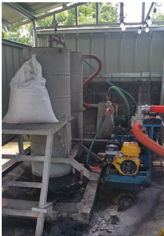
Figure 1. The Rice Husk Gasifier for Pumping Water.
